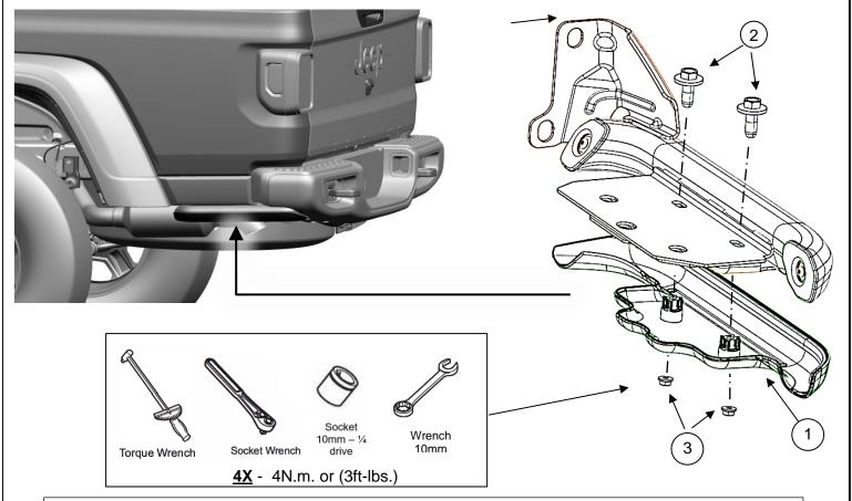
CAUTION: Over tightening fasteners can lead to component damage.
