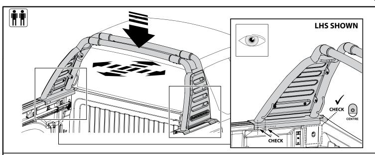
10. Using two people carefully lift the sports bar into position above the tub and slowly lower the Sports Bar Front Foot through the bed rail hole and lower the sports bar assembly onto the tub of the vehicle. Align the bar carefully and check that all drilled holes in the tub align with the holes in the bar.
