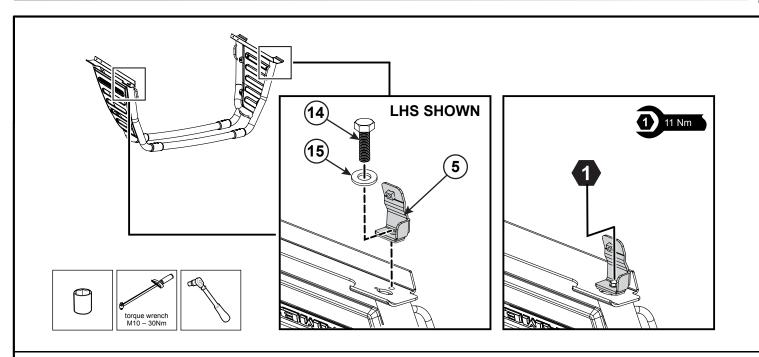
**4.** Assemble the Left Hand Side Front Foot (5) on tub rail bracket using Hex Head Bolt (14) and Washer (15). Slide a Joiner (7) over the ends of the Tubes and push both Legs (1),(2) through the Joiners into the top Tubes (4),(5). Align the holes in the Joiners with the threaded holes in the side legs and top Tubes and loosely secure with the Flanged Allen Bolts (11).
