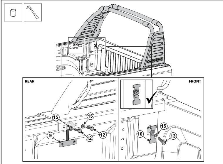
11. Loosely attach the bar to the bar to the front of the tub using the Front Foot Clamp (10), M8 Bolt (13) and M8 Washer (15). Attach the bar to the rear of the tub using the Rear Foot Clamp (9) and M8 Bolts (12) and M8 Washers (15) as shown.
