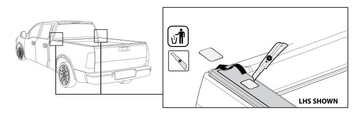
5. Using a knife carefully cut out the plastic insert at the front of the LHS and RHS bed rail caps to open the clearance holes for the front feet of the Sports Bar.
