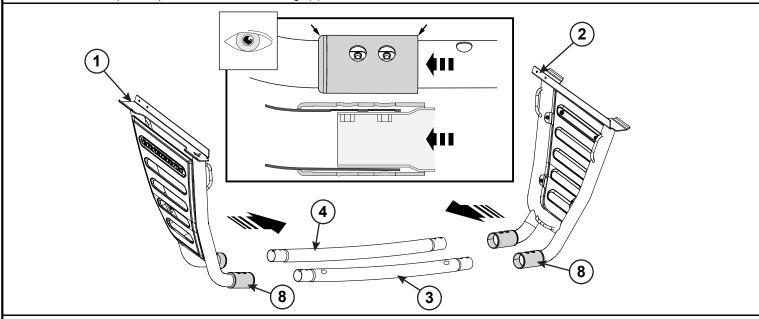
2. Assemble the Sports Bar by sliding the Front (3) and Rear (4) Tubes into the Side legs. Push the tubes into the Side legs and align the weld nuts in the Tubes with the holes in the plastic Joiners (8).
