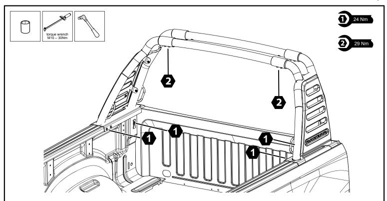
12. Centralize and check the final position and alignment of the bar on the tub. Tighten all M8 Bolts on the tub (13) and (12) to the recommended torque of 24Nm followed by the top bar Joiner Flanged Bolts (11) to a recommended torque of 29Nm.
