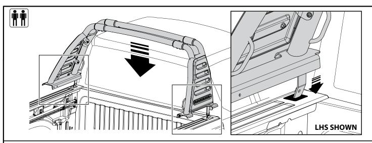
7. Using two people carefully lift the sports bar into position above the tub and slowly lower the sports bar Front Feet through the bed rail stake pockets and lower the sports bar assembly onto the tub of the vehicle.
