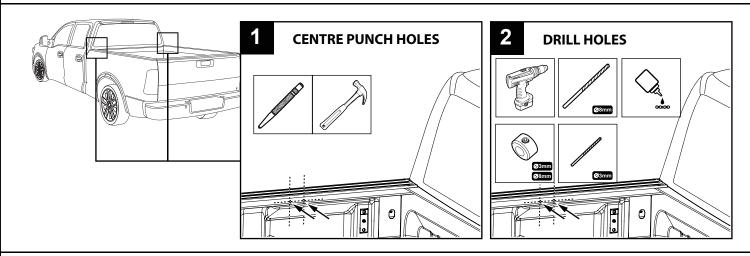
**9.** Centre punch the two marked hole positions and drill each hole with a 3mm drill bit then with an 8mm drill bit using a drill stop at 10mm. Coat exposed metal with rust inhibitor and clean up any metal swarf. Repeat for the RHS.
