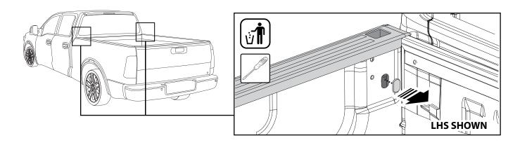
**6.** Remove and discard the LHS and RHS plastic side plugs from the Tub.
