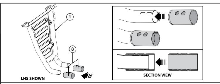
1. Assemble the Joiners (8) to the LHS Side legs (1) (by sliding the curved end over the bar first. Align the holes in the plastic Joiners with the slots in the bar as shown. Repeat the process for the RHS Side Legs (2).
