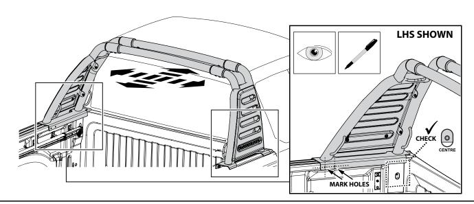
**8.** Align the bar carefully with the side rails and the front edge of the tub and position it in the precise position it will be attached to the vehicle. Check the threaded hole in the Front Foot is centred and mark the locations of the two rear holes onto the tub with a marker. Remove the Sports Bar.
