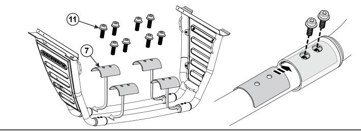
3. Slide the Joiner Plates (7) into the gaps between the plastic Joiners and the Tubes and align. Secure the Tubes together with the flanged bolts (11). Do not tighten.
