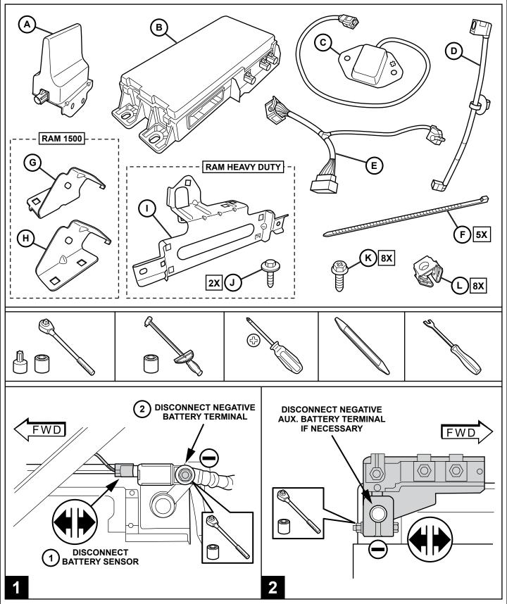
**FOR RAM 1500 FOLLOW** PAGES 2 THROUGH 7 NOTE: IT IS RECOMMENDED TO READ THE **INSTRUCTIONS THOROUGHLY BEFORE** FOR RAM HEAVY DUTY FOLLOW INSTALLING THIS ACCESSORY. PAGES 8 THROUGH 13 3 **RAM 1500 RETAIN ALL FASTENERS** FOR REINSTALLATION 5 6 **3X**
