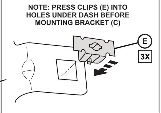
**NOTE: PRESS CLIPS (E) INTO HOLES UNDER DASH BEFORE MOUNTING BRACKET (C)**
