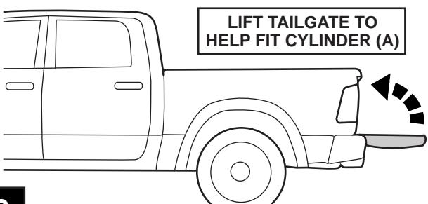
**LIFT TAILGATE TO HELP FIT CYLINDER (A)**
