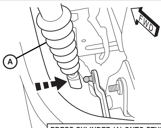
**PRESS CYLINDER (A) ONTO STUDS AT TOP AND BOTTOM**
