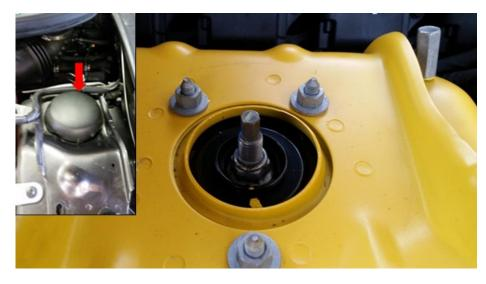
1. Locate the production strut caps and remove with a plastic trim tool. Verify there are 7-8 threads on the strut tower to install the new MOPAR Strut Caps.
