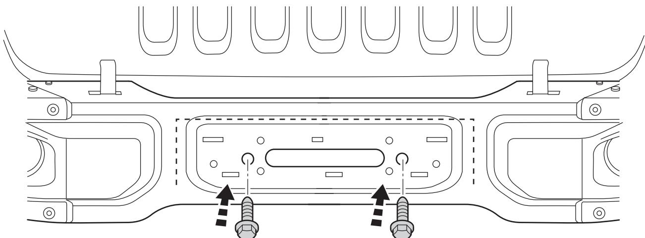
**NOTE: INSERT TEMPORARY BOLTS TO ALIGN PARTS**
