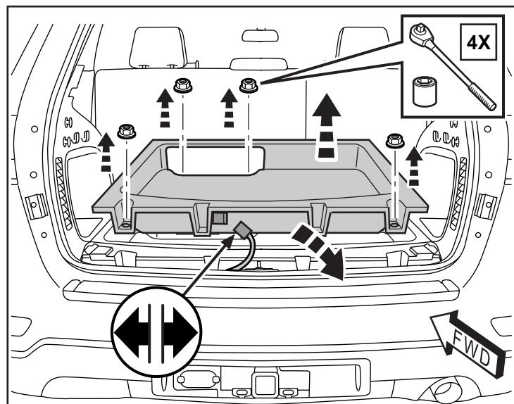
34. Remove three (3) fasteners as shown. Carefully pry back the lower trim panel on the driver side of the rear hatch area.
