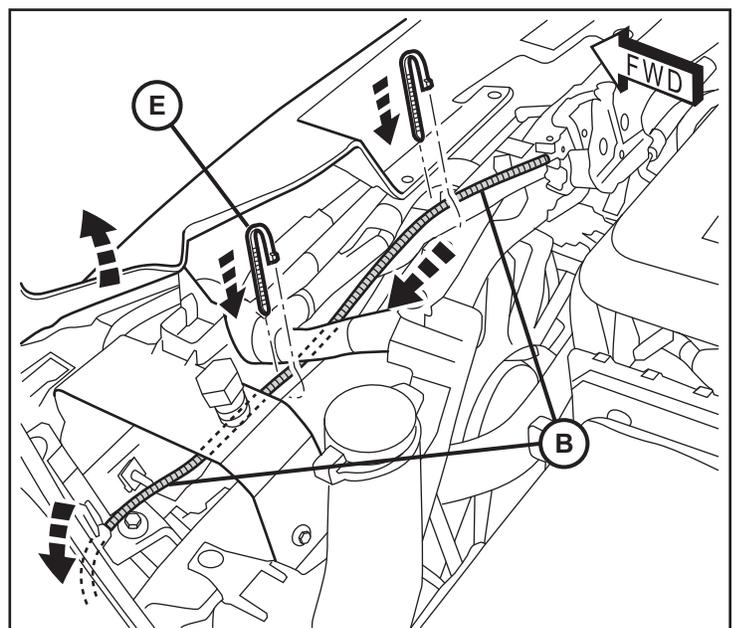
7. Route the switch harness (B) along the existing vehicle harnesses on the driver side and back towards the rear of the engine compartment. Tuck the harness behind the fuse box as shown.
