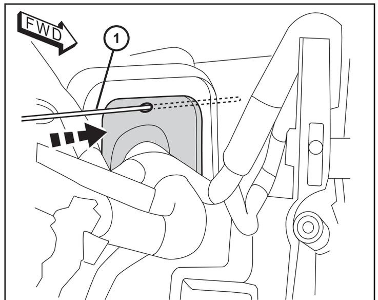
13. Secure the end of the harness to the fish wire with tape. Pull the end of harness (B) through to the inside driver footwell. Apply RTV sealant to the hood switch wiring convolute and pull the wiring into the nipple to seal the wiring at the nipple.
