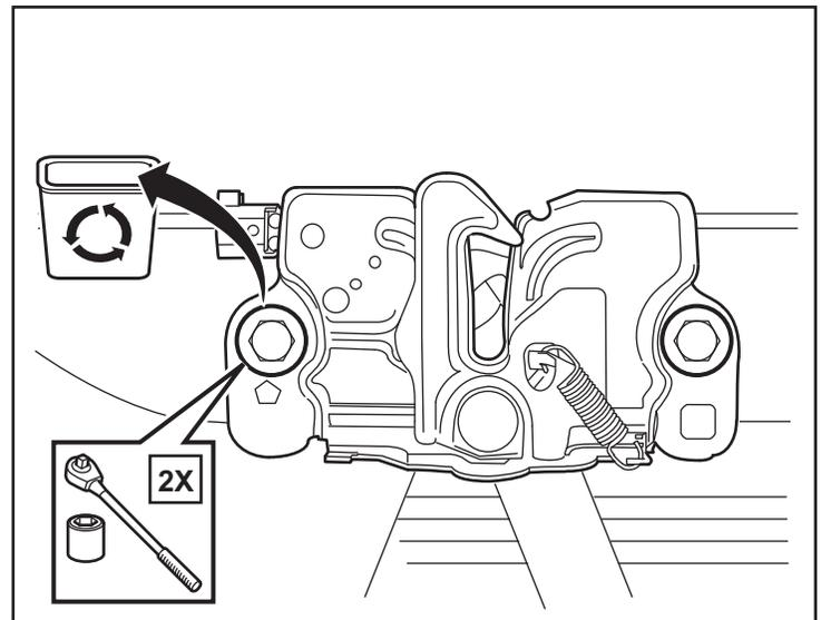
3. Carefully pry back the radiator cover panel. Disconnect and remove the hood latch release cable. Remove the hood latch assembly.
