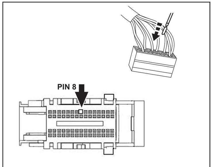
18. Reinstall the outer casing on the connector.
