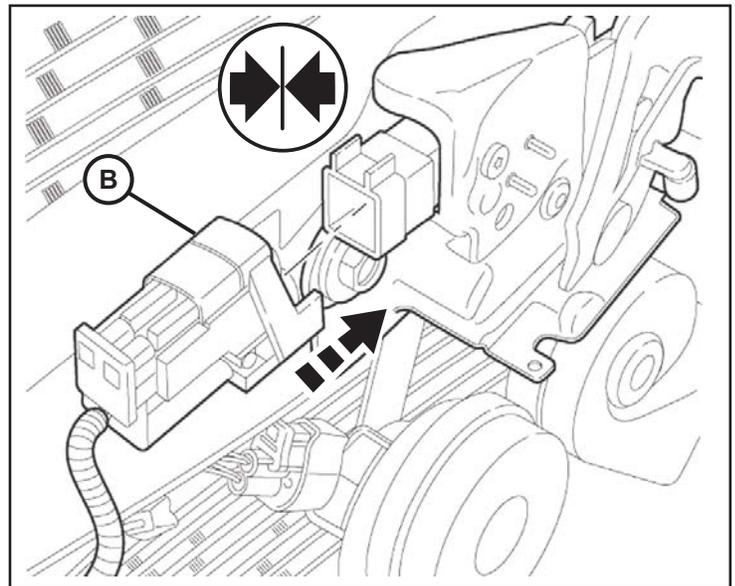
6. Carefully pry back the radiator cover panel. Route the switch harness (B) over towards the driver side along the existing vehicle harness. Feed the switch harness under the hoses and brackets as shown. Secure with cable ties (E).
