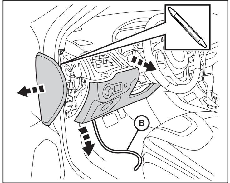
11. Remove two (2) fasteners from the hood release lever assembly and lower the assembly down under the dashboard.
