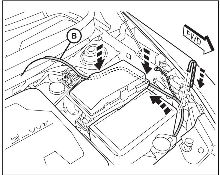
8. At the fender edge next to the battery, remove the existing ground wire hex nut. Position the ground ring terminal from the main harness (B) and reattach the nut to secure.
