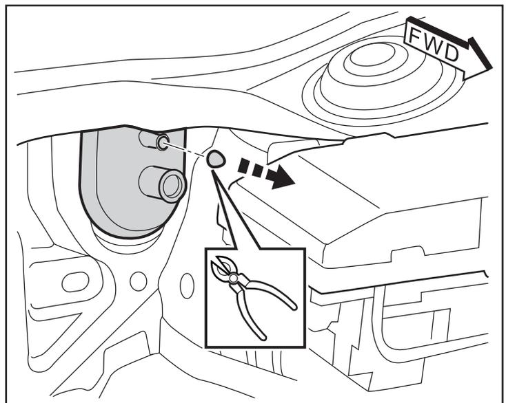
10. Carefully pry off the trim panel at the end of the dashboard on the driver side. Pry off the lower trim panel under the steering column. Pull the Switch Harness (B) through to the inside footwell.
