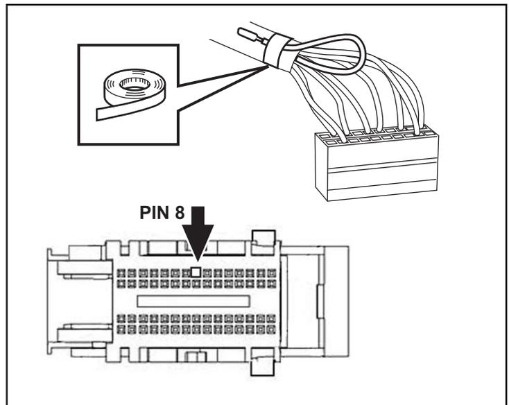
17. Insert the tab wire connector from switch harness (B) into Pin 8 on the connector.
