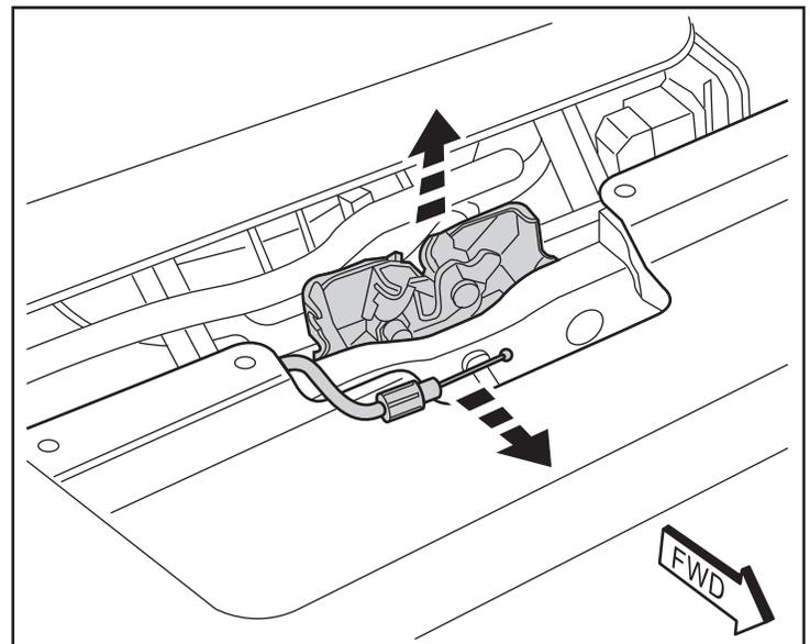
4. Reconnect the hood latch release cable to the back of new hood latch assembly. Position the new hood latch (A) with the alignment marks and secure with two (2) hex bolts. Tighten bolts to 9 Nm (80 in. lbs.)
