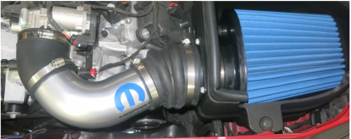
g) Install the assembly in the vehicle as shown. and tighten the Hose Clamps to 3.2Nm (28.3 in-lb)
