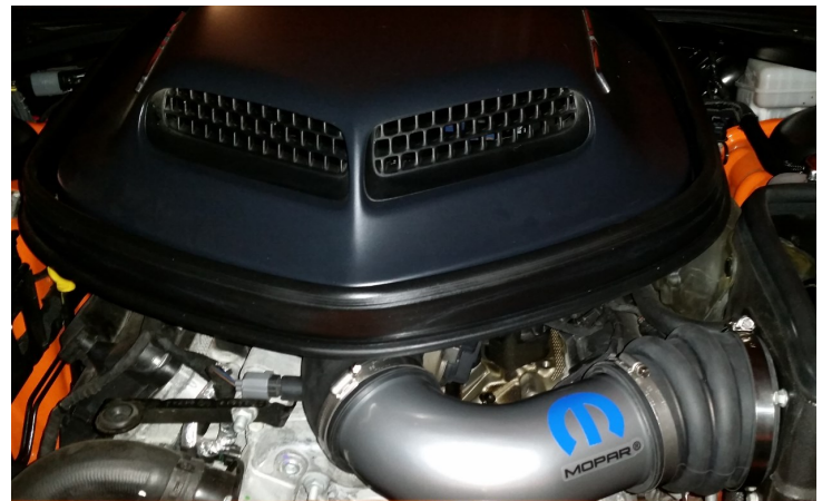
i) Reinstall the Shaker Scoop Assembly as shown on the next two (2) pages.
