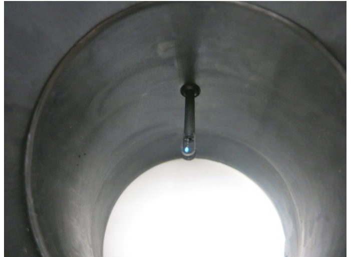
b) Make sure the IAT sensor is inserted all the way into the throttle body Coupler as shown.
