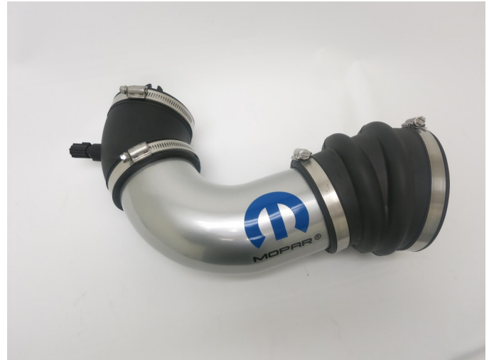
f) Slide the Elbow Hose on the opposite end of the MOPAR Inlet Tube as shown. Do not tighten the hose clamps.
