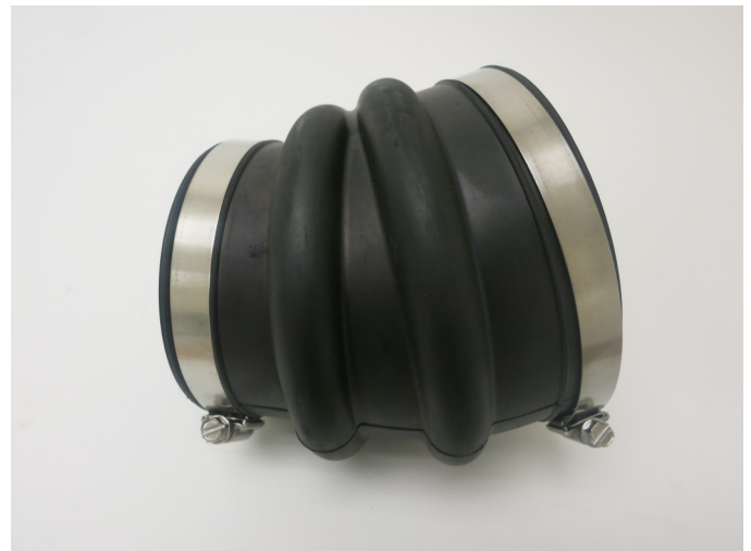
d) Install the one (1) 4.00" and one (1) 5.00" hose clamp on the elbow Hose. (Clamp alignment not critical)
