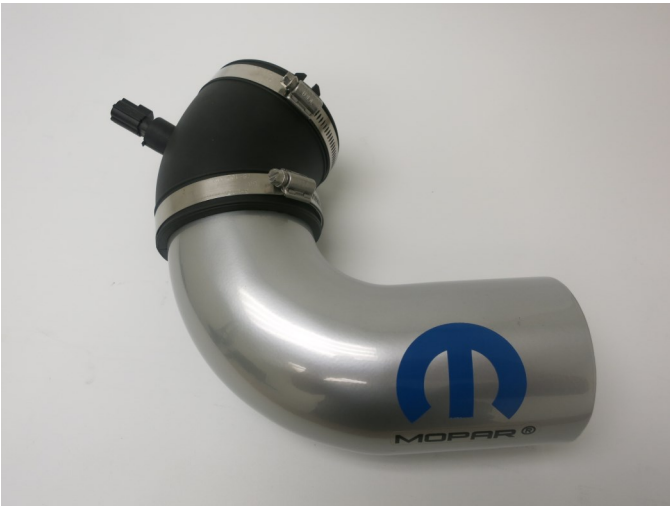
e) Insert the MOPAR Inlet Tube into the throttle body Coupler as shown. Do not tighten the hose clamps.
