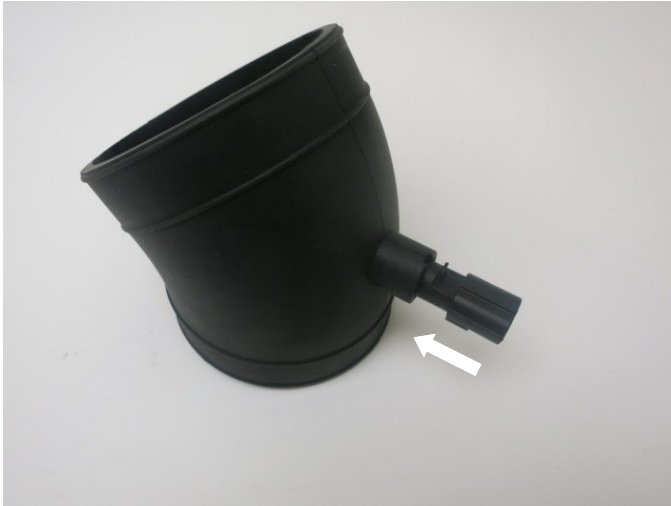
a) Insert the IAT sensor into the throttle body Coupler as shown. Orient the sensor probe relative to the notched lip.
