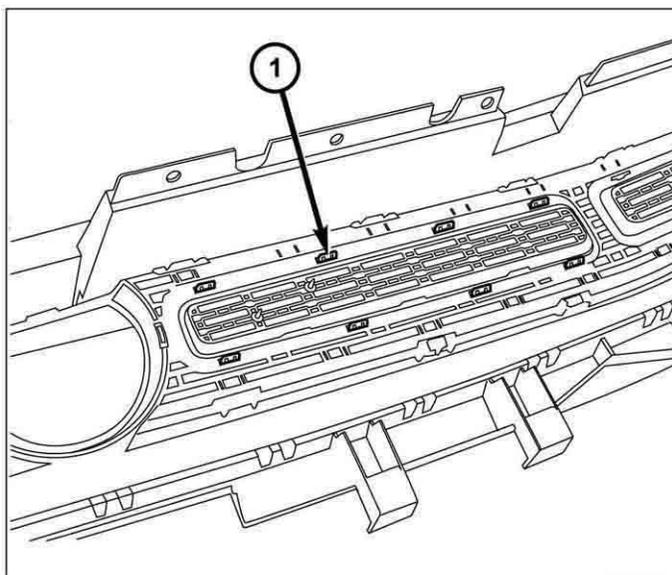
19. Insert the driver side trim ring (1) into position in the fascia as shown.
