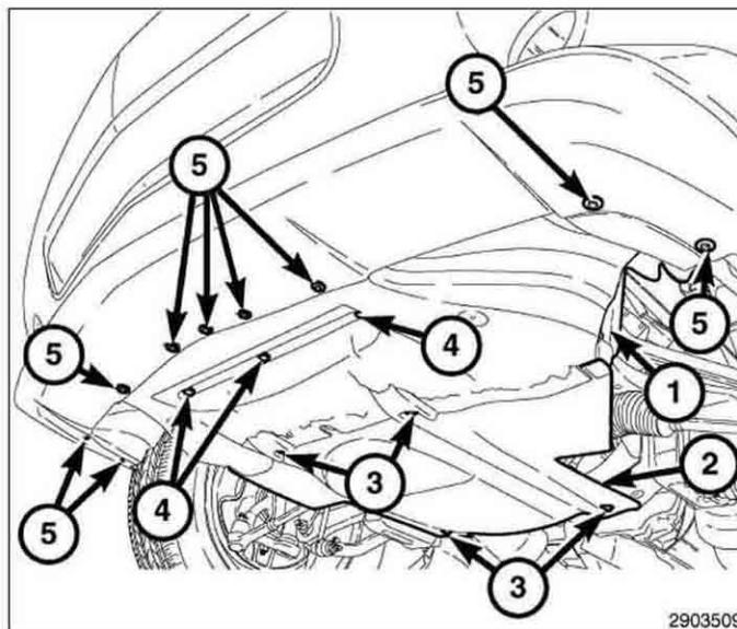
34. Using a new rivet and rivet gun, install the rivet (1) securing the splash shield to the fender.
