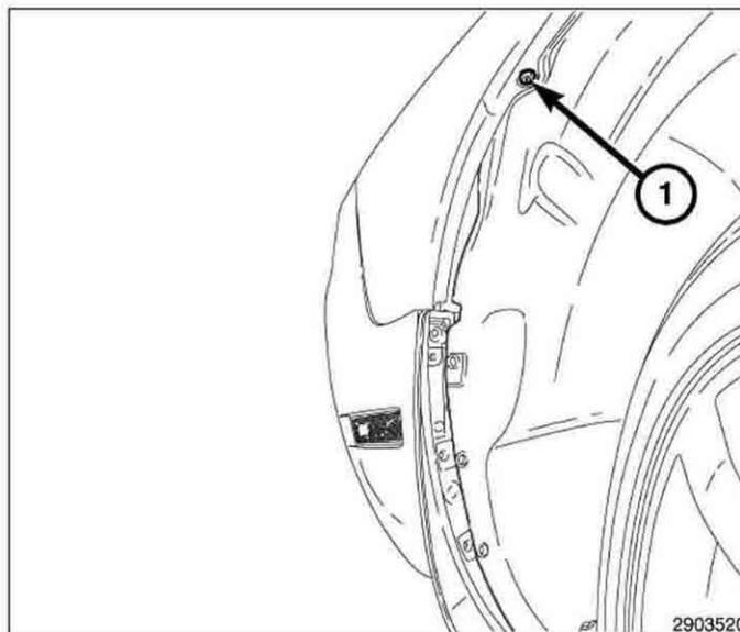
35. Using new rivets and rivet gun, install the three rivets (1) securing the splash shield to the fascia and discard.
