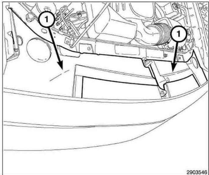
30. If equipped, connect the fog lamp's main harness (1, 2). The harness will be located near the bottom of the windshield washer solvent container.
