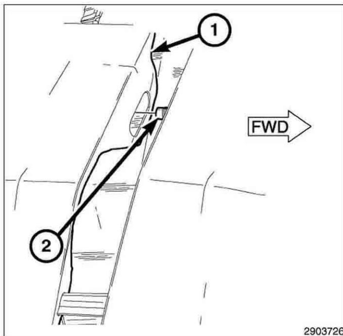
25. Align the fascia fender tabs into the fender retaining slots and push the fascia (1) inward to engage.
