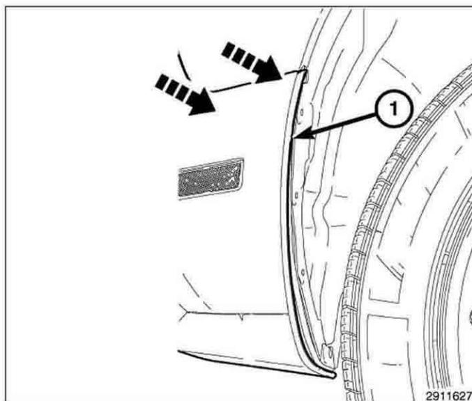
26. Install the three upper fascia to upper radiator cross-member fasteners (1) on the right hand side of the vehicle.
