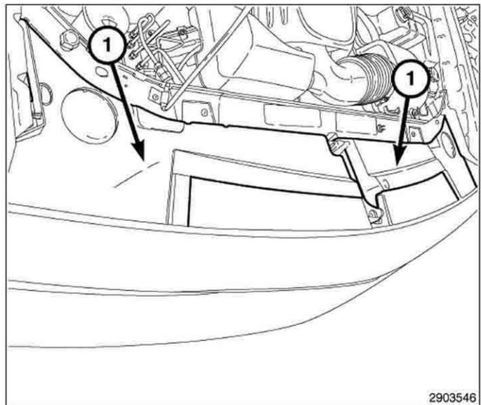
13. Remove the nut (1) securing the upper front fender to the upper fascia. Save for re-use.
