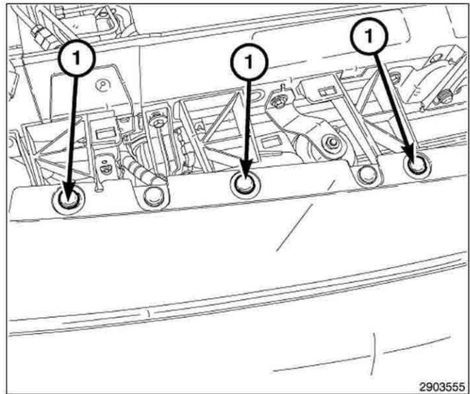
15. Carefully pull outward on the fascia (1) from the wheelwell to disengage the fascia fender tabs from the fender retaining slots.
