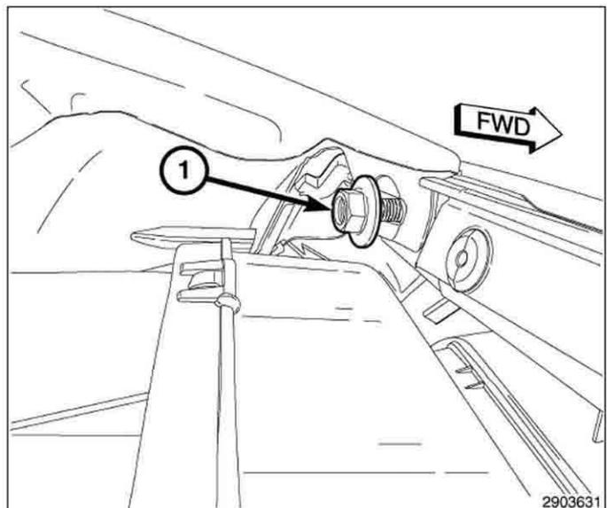
14. Remove the three upper fascia to upper radiator crossmember fasteners (1) on the right hand side of the vehicle. Save for re-use.
