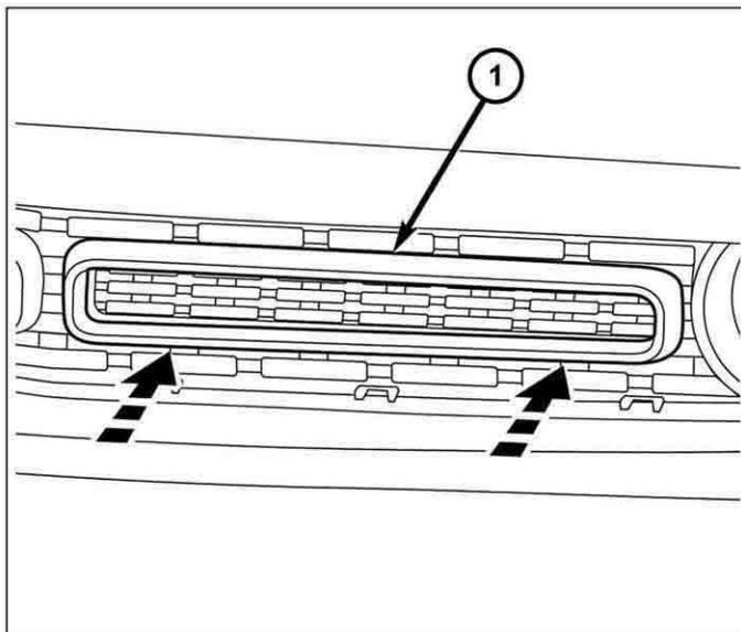
20. Carefully snap the eight mounting clips (1) into position to secure the driver side trim ring.
