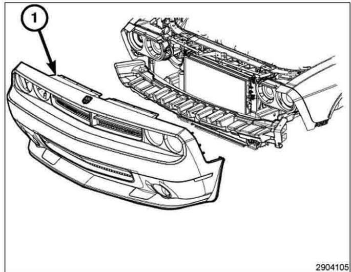
17. Place fascia on a clean work surface. From the rear, carefully release the eight clips (1) holding the driver side trim ring.
