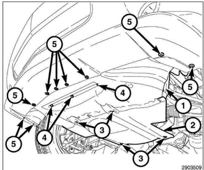
9. Remove one nut (1) and one bolt (2) securing the lower portion of the fascia to the inner fender (3). Access the nut (1) through the opening between the wheelhouse splash shield at the fascia. Save for re-use
