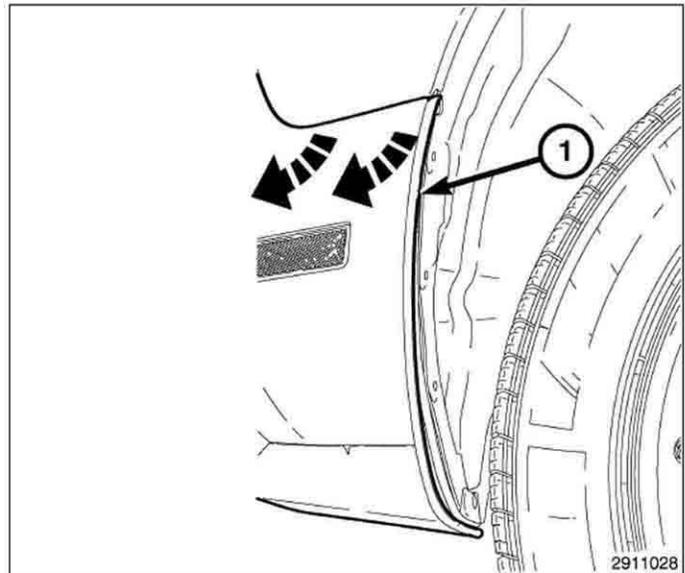
16. With the help of an assistant, pull the fascia (1) from the front and remove the fascia (1) from the vehicle.
