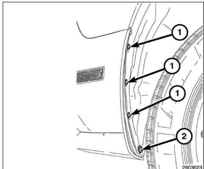
6. Remove the rivet (1) securing the splash shield to the fender and discard.
