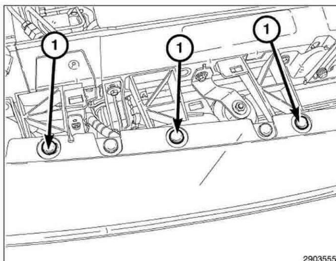
27. Install the nut (1) securing the upper front fender to the upper fascia. Tighten the nut (1) to 3 N-m (26.5 in. lbs.).
