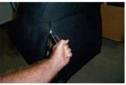
6. Re-hook the bottom of seat back panel
