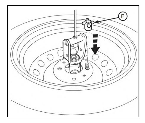
10. Raise the tire with the lug nut wrench (**B**) until the effort increases and you hear a snap noise. Then check the transparent window for the cable end position.
