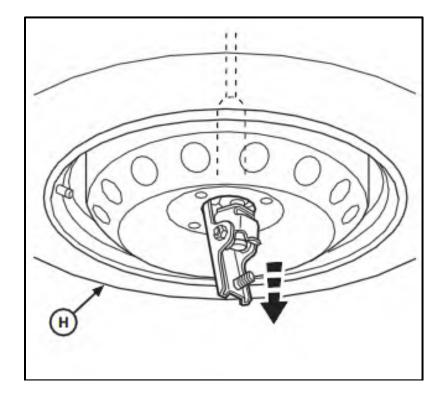
9. From the top side of the spare tire, be sure the threaded stud on the retaining shoe passes through one of the wheel lug hole. Install the wheel lock knob (**F**) and hand tighten securely.
