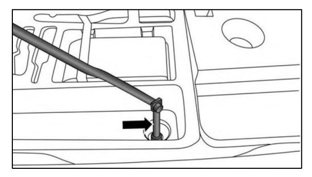
8. Lift the spare tire (**F**) into position with the stem side down. Slide the retaining shoe through the center hole as shown.
