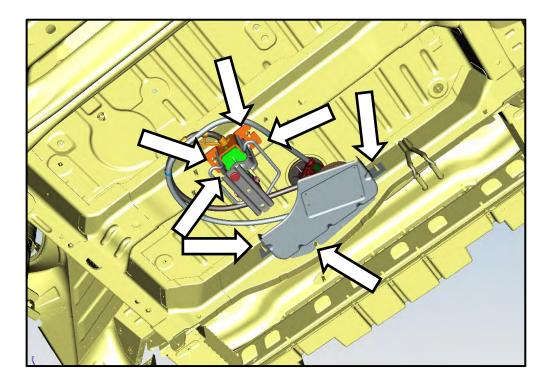
6. Install the two wheel brackets (B). Fasten with two M8 nuts each (A) and torque to 25 Nm.
