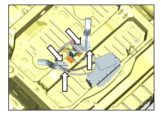
7. Extend the winch cable to allow room for the tire. Use the Lug nut wrench (B) to extend the cable.
