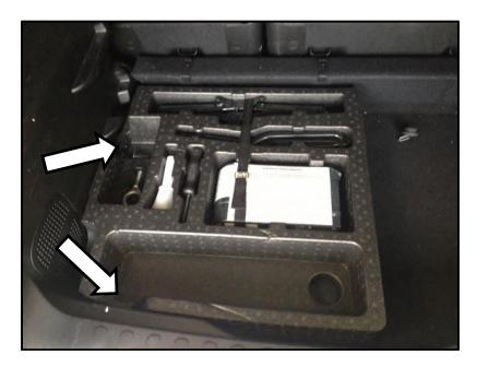
3. Move carpet to gain access to the body plug. Remove the plug and discard.
