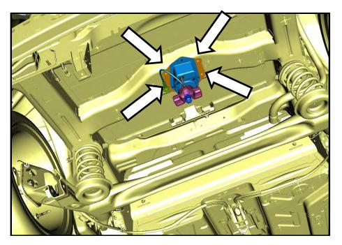
5. Position the Left and Right Hand Brackets (B, C). Fasten with two M8 bolts (F) each, then torque to 20 Nm.
