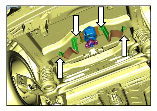
6. Position the heat shield then install four Stamped Nuts (E).
