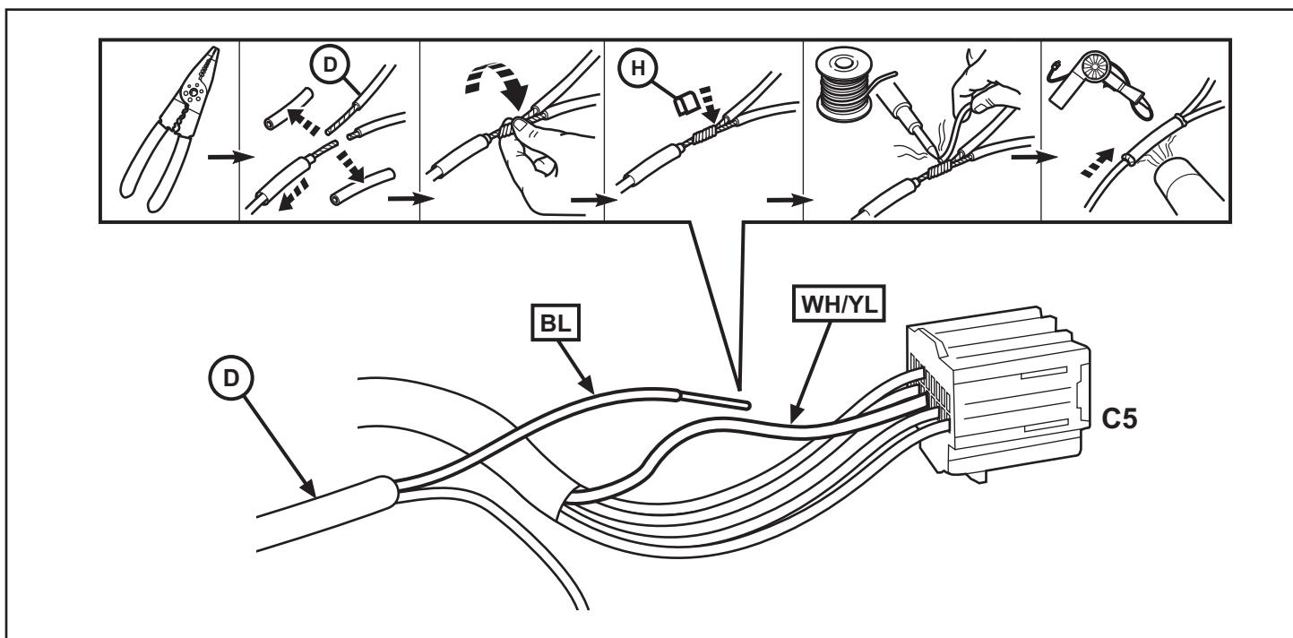
17. Wrap the harnesses with electrical tape to secure the new wiring as needed. Reconnect the plugs to the fuse box. Carefully press the fuse box back into position. Be sure not to crimp any of the harnesses.
