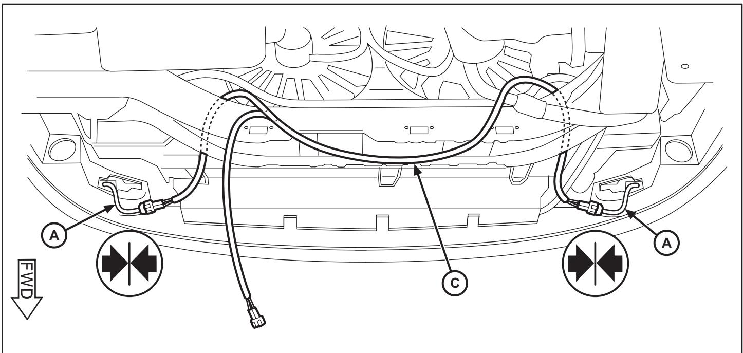
11. Secure the lamp harness with cable ties along the existing harness under the front fascia as shown. Route the harness pigtails up through the top of the engine compartment.
