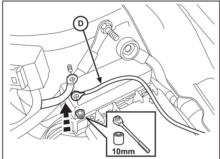
19. Locate and remove two (2) 10mm inside the edge of the fender next to the fuse box.
