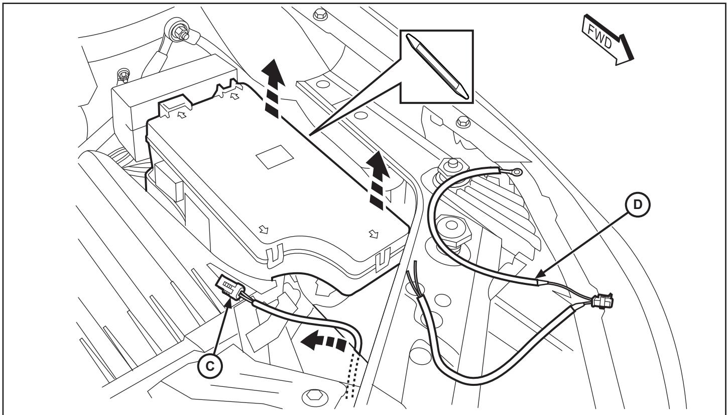
14. Locate and disconnect the two plugs shown (C7 and C5). Carefully pull the plugs out away from the fuse box in order to access the wiring harnesses.
