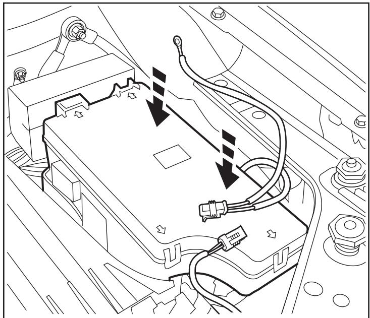
18. Locate the ground wire behind the fuse box. Remove one (1) 10mm nut and install the ground eyelet from the power harness (D). Reattach the ground wire.
