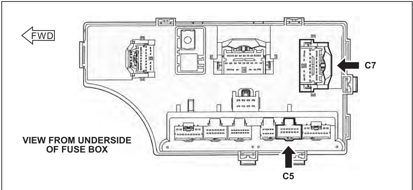
15. Carefully cut away some of the insulation and locate the pink/light blue wire in the C7 plug harness. Splice the red wire from the new power harness (D) to the pink/light blue wire.
