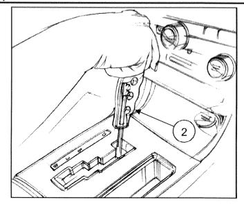
5) Cover with protective mat and tap shifter into place using rubber mallet. Tap until you feel the piece "bottom out".
