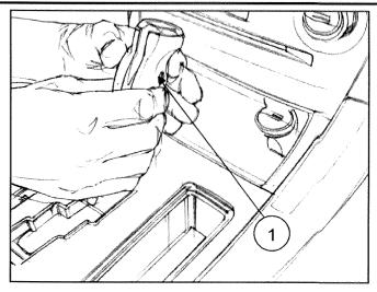
8) Install 3 phillips screws with screwdriver. Torque screws to 12in.lbs. +/- 2in. lbs.
