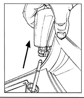
4) Place the Pistol Grip shifter center piece on to shaft.
