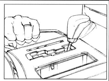
2) Using needle nose pliers, pull retainer clip from bottom front of shift collar.
