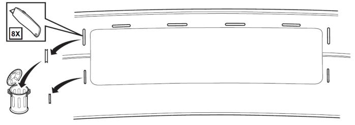
9. Cut out center bezel opening according to scribed area as shown. Discard cut out portion.
