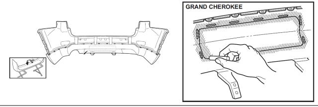
7. Drill starter holes for tab openings according to scribed areas as shown. Use a 1/8" (3.4mm) bit for the top six slots and a 3/32" (2.3mm) bit for the lowest two slots. Be sure to drill both ends of the slots.
