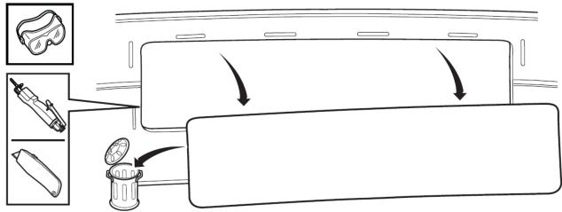
10. Press bezel into bumper opening. Be sure all tabs are firmly pressed in and secure with (2-4) spring clips as shown.
