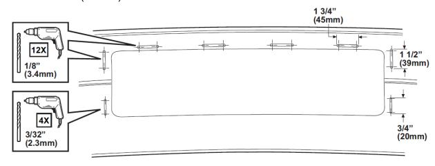
8. Cut through remaining area of tab openings with a utility knife according to scribed areas as shown. Discard cut out portions.
