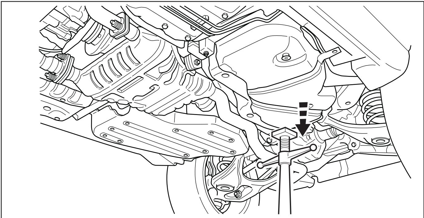
9. Install LH Fuel Tank skid plate using (1) 13mm and (3) 15mm support bolts from around fuel tank.
