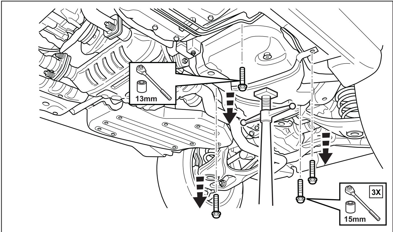
8. Carefully lower jack stand from beneath the fuel tank. Fuel tank will sag slightly, but remain supported to vehicle.
