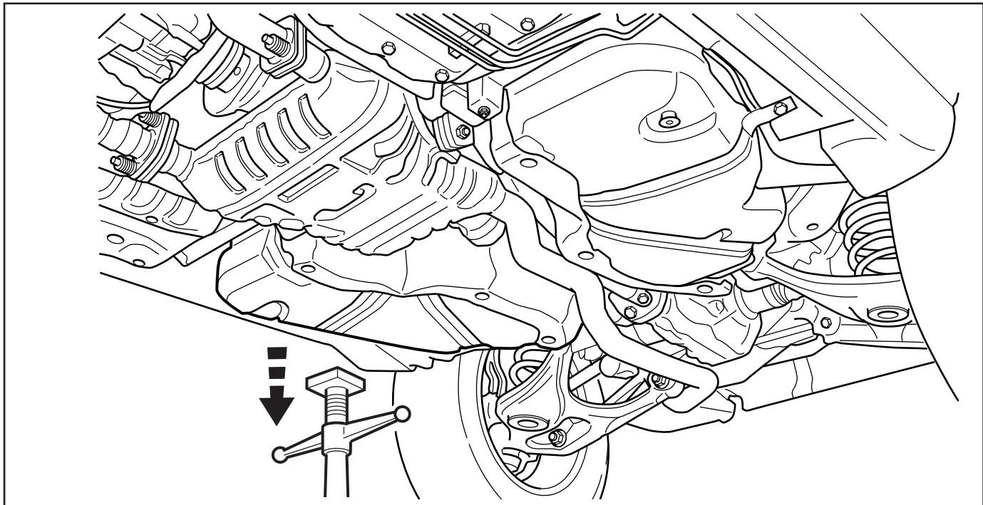
5. Install RH Fuel Tank skid plate using (1) 13mm and (3) 15mm support bolts from around fuel tank.
