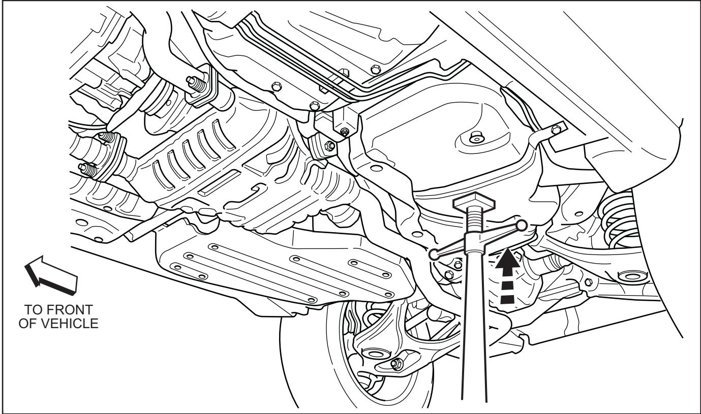
7. Remove (1) 13mm and (3) 15mm support bolts from around fuel tank.
