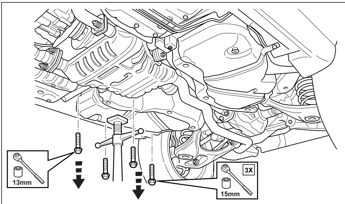
4. Carefully lower jack stand from beneath the fuel tank. Fuel tank will sag slightly, but remain supported to vehicle.
