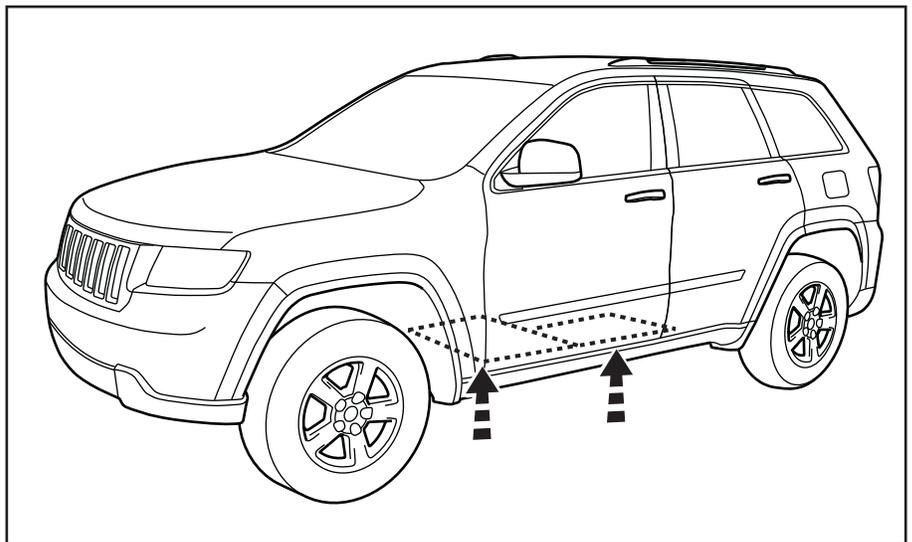
3. Remove two metal cross braces from underside of vehicle as shown. Remove the plastic cover panel from the driver side of the vehicle.
