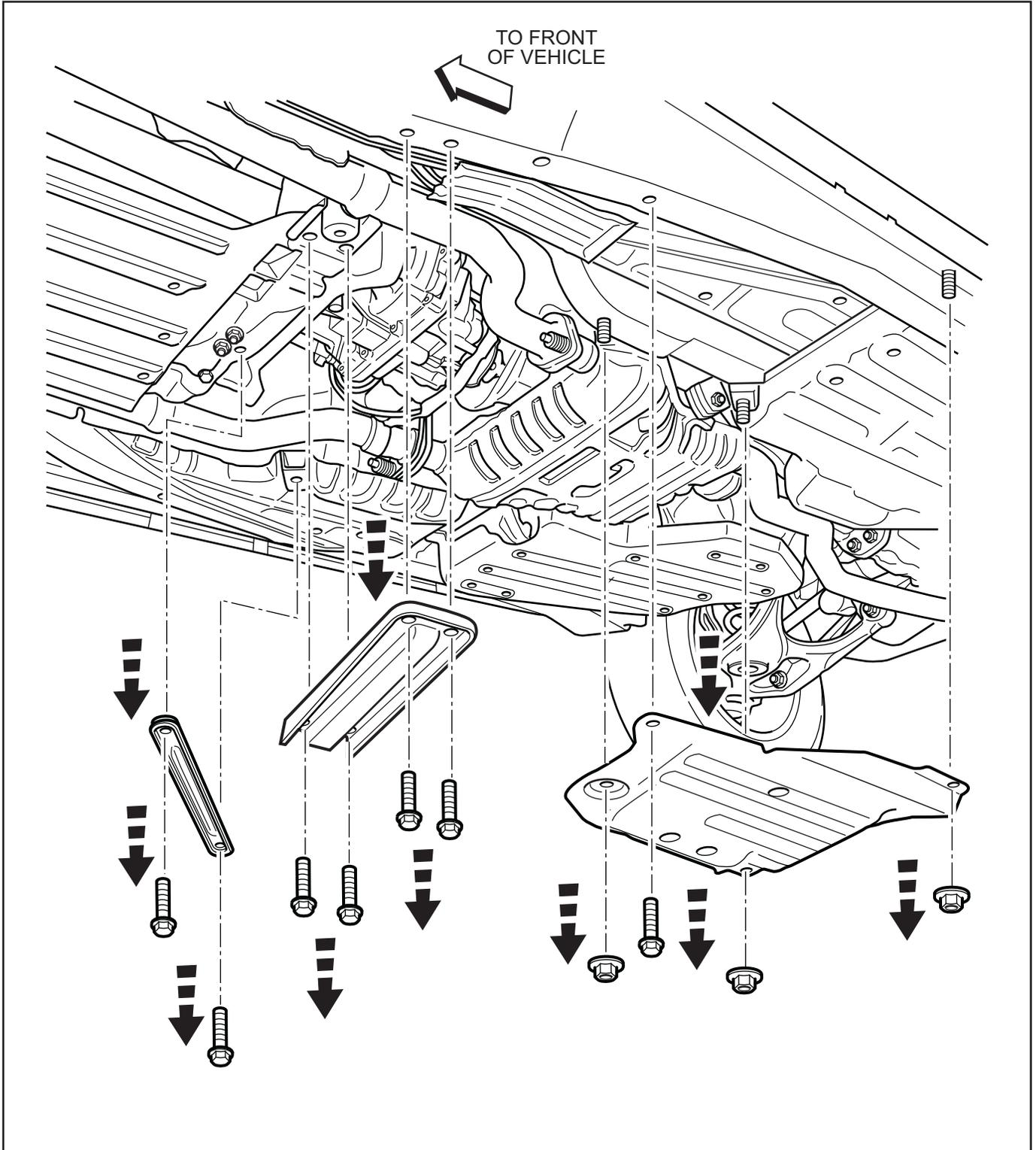
4. Fasten Fuel Bundle Skid Plate (B) into position as shown using (3) 13mm nuts provided. Tighten to 20 Nm (15 ft. lbs.)
