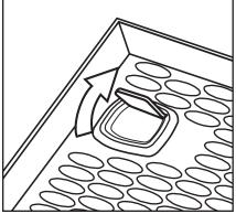
3. OPTION: If cargo tray tie down openings are needed, carefully use a knife to cut the flap opening as shown.
