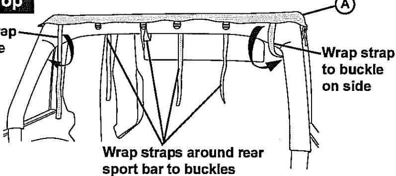
Wrap the straps on the rear of the Sunbonnet around the rear sport bar. Thread them through the buckles. Wrap the two (2) outside straps around to the buckles on the side.
