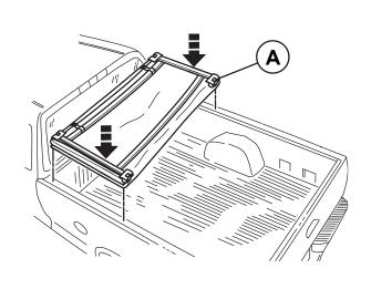
Place the cover assembly on the top of the truck bed next to the cab.
