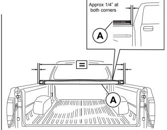
Line up to front of bed first. Center the cover assembly on the truck. Position the cover assembly so the gaps on all sides are equal.
