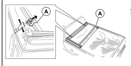
The cover has retaining straps with quick-release buckles to keep it from being damaged when bulk hauling or when it is not on the vehicle.
