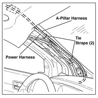
**9)** Secure power harness to existing A-pillar harness with two tie straps.
