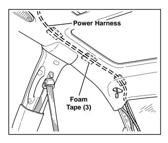
**8)** Using foam tape, secure power harness to the inside of headliner as shown.
