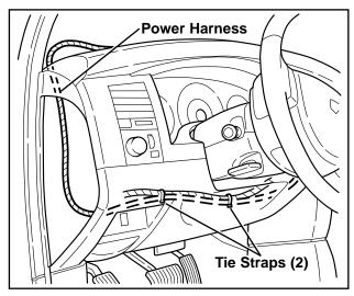
2) Route power harness up inside the I/P as shown. Keep it between left A-pillar and I/P top cover.
