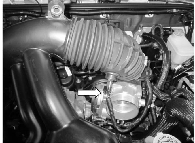
**f)** With the two M6 bolts removed, lift the air inlet hose up to reveal the IAT sensor and harness.
