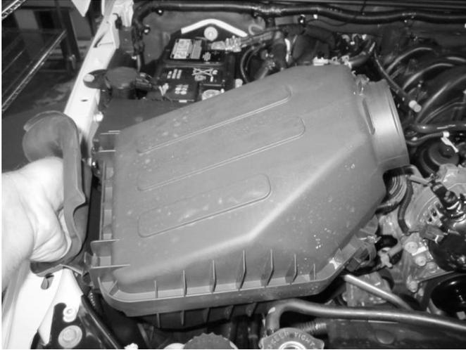
i) Remove the air box by placing a firm grip on it and pulling upward (there are 3 grommets that hold this box in place).
