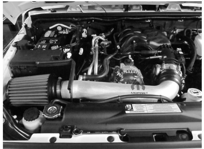
**n)** MOPAR Cold Air Intake installed on vehicle without the engine cover.
