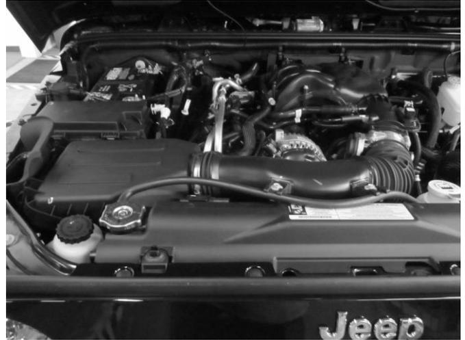
b) Lift the engine cover and remove it from the engine bay.
