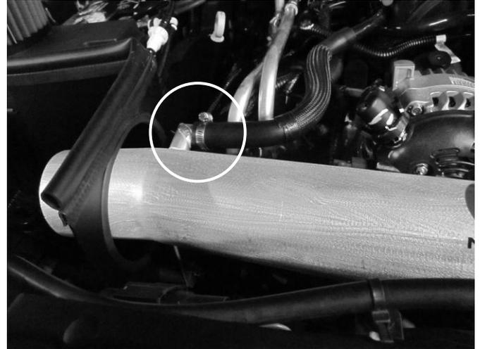
**l)** Attach the stock breather hose to the breather tube on the intake tube and secure with the supplied #12 hose clamp.
