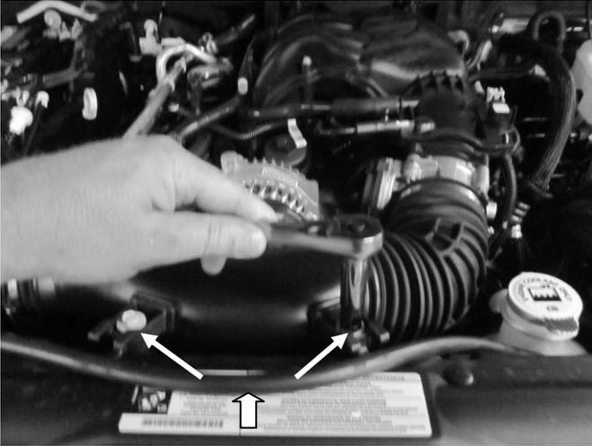
**e)** Loosen and remove the two M6 bolts securing the air inlet hose to the radiator support. Unclip the radiator overflow hose from the air inlet hose.
