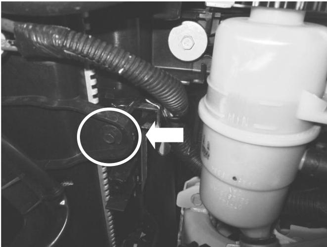
k) Loosen and remove the M6 screw securing the radiator fan shroud. The bolt will be reused in the later steps.
