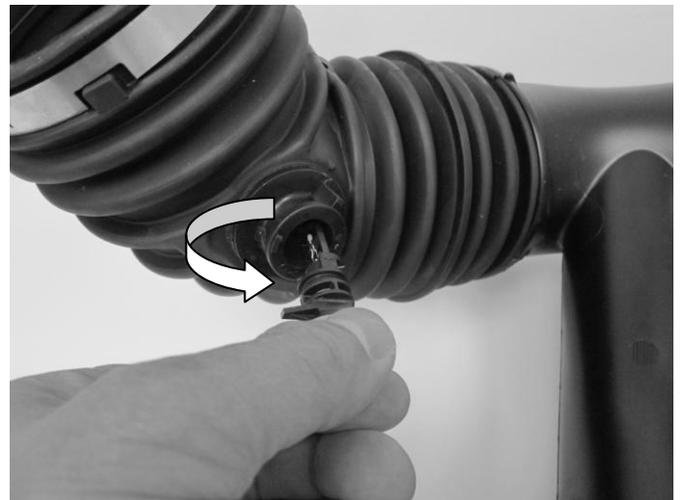
l) Remove the IAT sensor from the factory air inlet tube. Gently twist and pull out the sensor.
