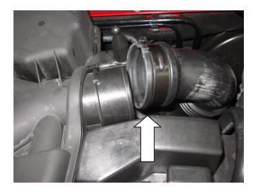
g) Loosen the clamp on the hose to the air box and detach the hose from the air box.
