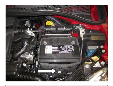
c) Disconnect both battery terminals and remove the battery stay on the battery tray.
