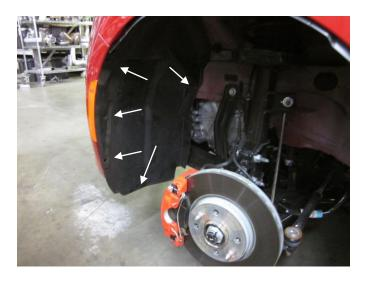
v) Install the screws securing the plastic fender liner to the front bumper; Install the wheel back on the vehicle, torque the lug bolts to manufacturer's recommend specification.
