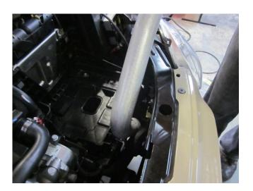
g) With care, guide the Cold Air Inlet tube through the space between the battery tray and radiator hose, down to the lower inner bumper area. Note: It's a good idea to keep the plastic sleeve over the tube to protect the finish from being scratched.
