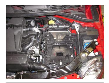
d) Remove the battery from the engine bay and set it aside.
