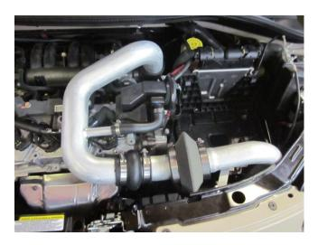
q) Attach the vent hose to the main air inlet tube with supplied #10 mini hose clamps as shown.
