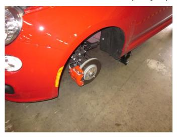
a) Properly jack up and support the vehicle and remove the front driver side wheel.
