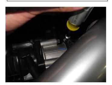
r) Tighten all hose clamps on the throttle body and main air inlet tube after all tubes have been adjusted to have ample clearance.
