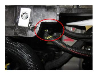
e) Unclip the lower harness retainer with a pair of needle nose pliers to release it from the holder.
