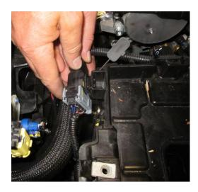
t) Clip the wiring harness holder back onto the battery tray.
