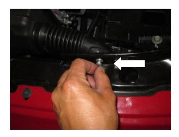
f) Loosen and remove the M6 bolt securing the air duct to the radiator support.
