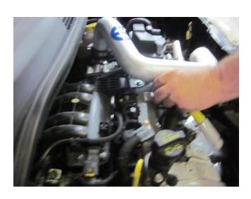
k) Insert the Main Air Inlet Tube into the 90 degree elbow hose on the throttle body. Do not fully tighten the hose clamp.
