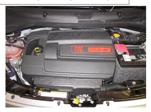
b) Factory air intake system. Gently pull up on the engine cover and remove it from the engine bay. The engine cover will not be re-installed. We recommend that you do not discard the engine cover.
