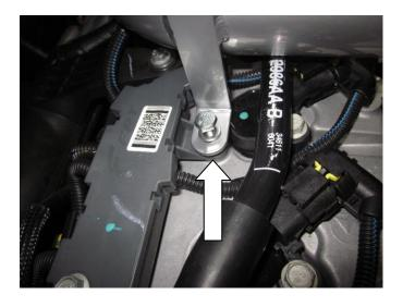
I) Line up the support bracket on the Main Air Inlet Tube to the threaded hole on the valve cover and attach with supplied M6x25mm bolt and nylon spacer. Note: Place the nylon spacer between the support bracket and the valve cover.
