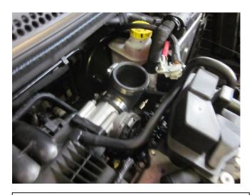
j) Attach the 90 degree elbow hose to the throttle body with supplied #40 hose clamps. Do not fully tighten the hose clamps at this point.
