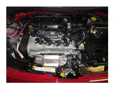
i) Lift the air box up and out of the engine bay. We recommend that you do not discard the factory air box.
