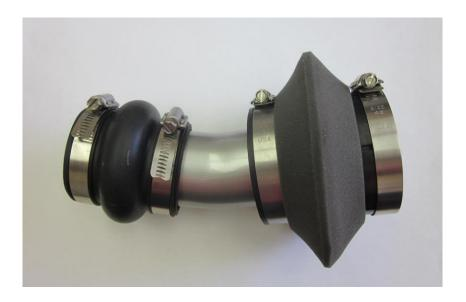
m) Assemble the hump hose, Transition tube, and Air-Bypass valve in the order shown in the picture. Keep the clamps loose as adjustments may be necessary during fit up.
