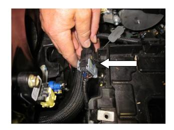
d) Unclip the wiring harness holder from the battery tray with a gentle pull.
