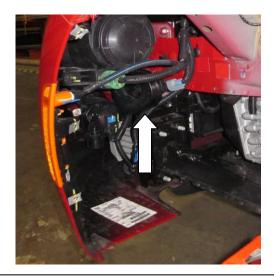
c) With the screws removed the fender liner can be peeled back to gain access to the horn. Loosen the M8 bolt and rotate the horn so the opening of the horn is facing forward. Tighten the M8 bolt after completion.
