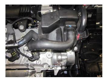
p) Attach the factory vent hose removed in page 4 step h) to the factory breather canister as shown. .
