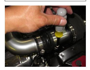
s) Tighten all hose clamps on the hump hose and air bypass valve after all tubes have been adjusted to have ample clearance.
