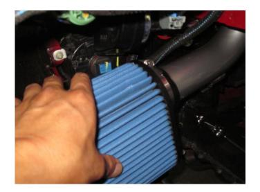
u) Install the Dry Flow air filter to the Cold Air Inlet tube and tighten the hose clamp. Make sure the air filter is not in contact with any adjacent parts.
