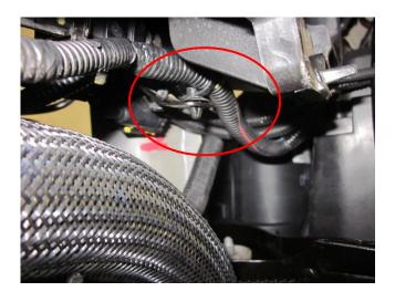
f) Move the harness to the opposite side of the holder and clip the retainer to the holder as shown. This will provide more clearance for the Cold Air Inlet tube.
