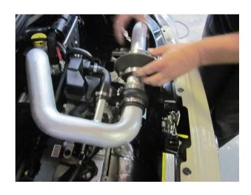
o) Attach the other end of the assembly to the to the Cold Air Inlet tube. Do not tighten the hose clamp at this point.
