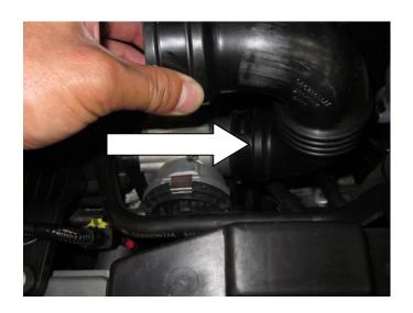
j) Lastly, loosen the hose clamp on the air inlet tube to the throttle body and remove the tube.
