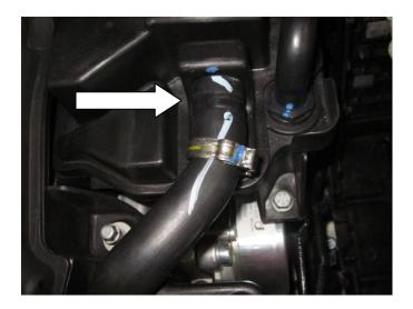
h) Use a pair of pliers to un-fasten the hose clamp at the breather canister and remove the vent hose. Please keep the vent hose as it will be reinstalled later.
