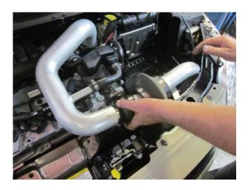
n) Attach the assembly from step m) to the Main Air Inlet tube. Do not tighten the hose clamp at this point.
