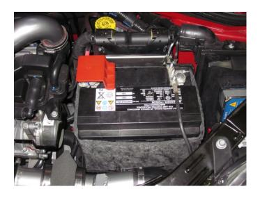
w) Install the battery and attach the battery stay to the tray.
